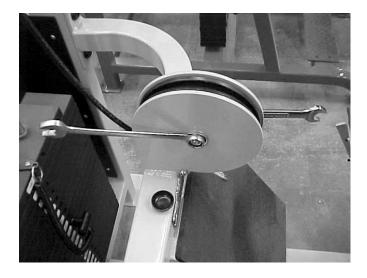
Figure 6. Removing the pulley bolt.
